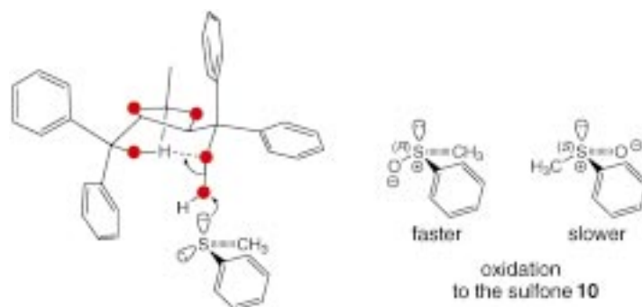
Fig. 4. Mechanistic model rationalizing preferential formation of (S)-methyl phenyl sulfoxide ( 9 ) from methyl phenyl sulfide, and TADOOH 3 , as well as faster 'overoxidation' to the sulfone 10 of (R)-sulfoxide 17 )
